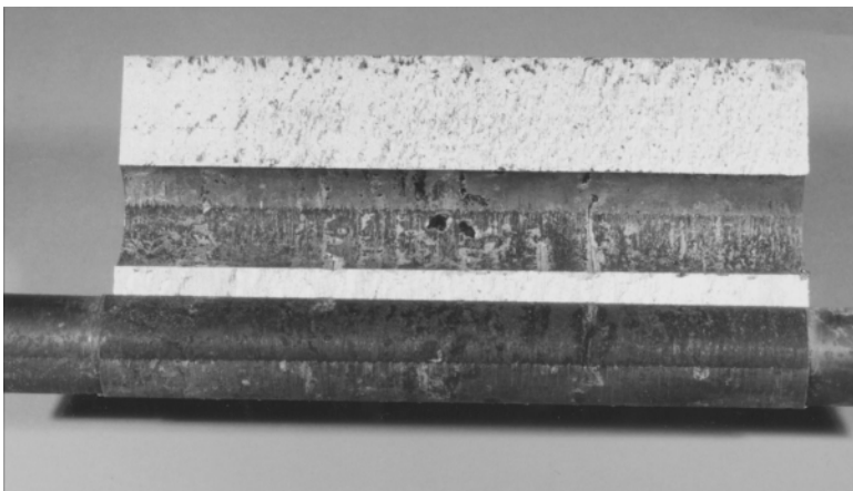
11.12 Steel-aluminium plain insert after pressure testing.
