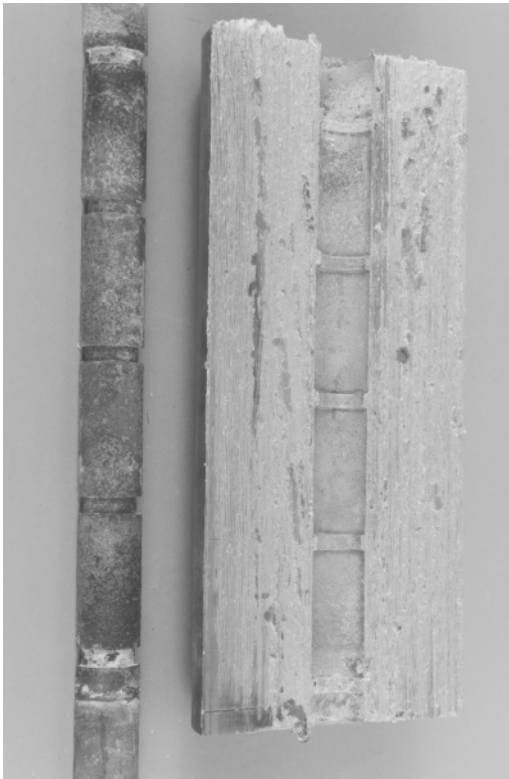
11.14 Plain steel insert with regular throttling after pressure testing.
