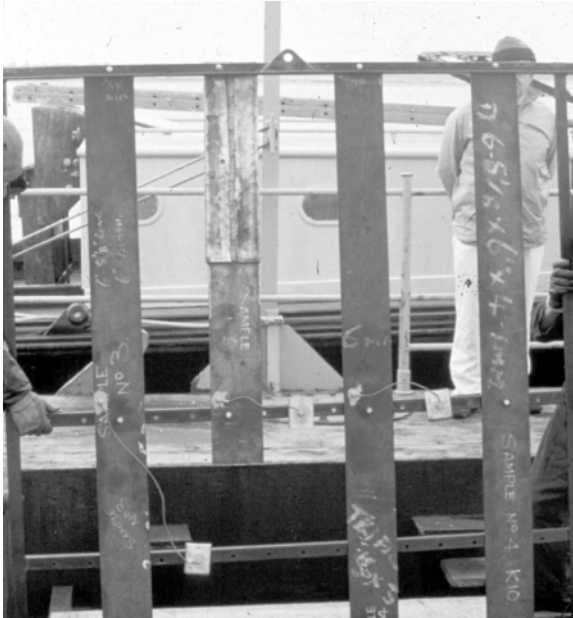
5.3 Cathodically protected steel, CuNi90/10 partially sheathed steel and CuNi 90/10 panels and a freely exposed copper nickel panel prior to immersion from a raft, UK.
